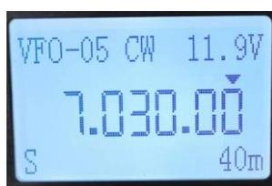
Press the knob on the right to switch the step frequency between 100KHz, 1KHz, 100Hz and 10Hz (press the knob for more than 2 seconds to change the step frequency in the opposite direction). When the step frequency is changed, there is a small triangle mark above the corresponding frequency display position on the LCD screen. If you press the big knob in the MEM state, it will get into the VFO mode.
