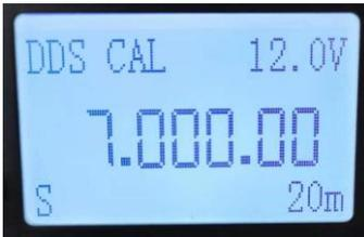
At this time, use a frequency meter to detect the frequency of the TEST point on the PCB board (between IC4 and IC5), turn the knob on the right side of the radio panel to adjust the frequency until the frequency meter displays 7.000.00MHz, press the M/V/S button for about 2 seconds Just exit.
