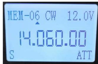
The ATT button is on the back of the radio. Press this button. The radio's high frequency gain is attenuated by about 15dB, and the LCD screen will display the word ATT.
