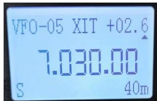
Tap this button once to enter or exit the receive fine-tuning and transmit fine-tuning (RIT and XIT) functions. At this time, the upper right of the LCD screen will display RIT or XIT and the amount of fine-tuning. After entering the fine-tuning state, press the right tuning knob to switch between receiving fine-tuning RIT and transmitting fine-tuning XIT.
