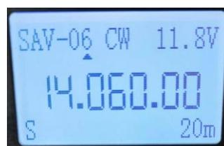
Press the M/V/S button for more than 2 seconds to store the current frequency and mode in the current storage unit. The word Sav-\*\* will be displayed in the upper left corner of the LCD screen. **Everytime the radio powered on,last saved memory of band, frequency and mode will recall.**
